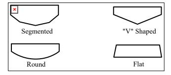
2. A hull which has no lateral side-to-side breaks, discontinuities, or steps in the wetted surface running at more than a 15° angle with the keel (in bottom view).
