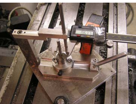
Setting Blade Radius Location from Shaft Center
