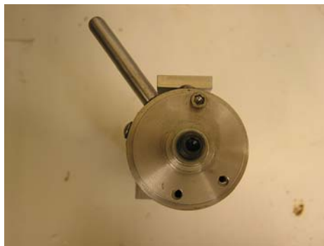
The index disk showing the offset holes
